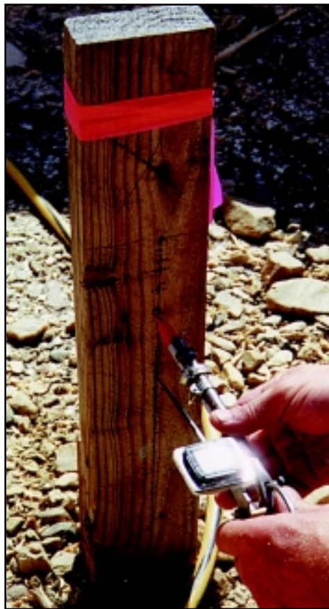
Use a benchmark to set the level bubbles for consistency.
