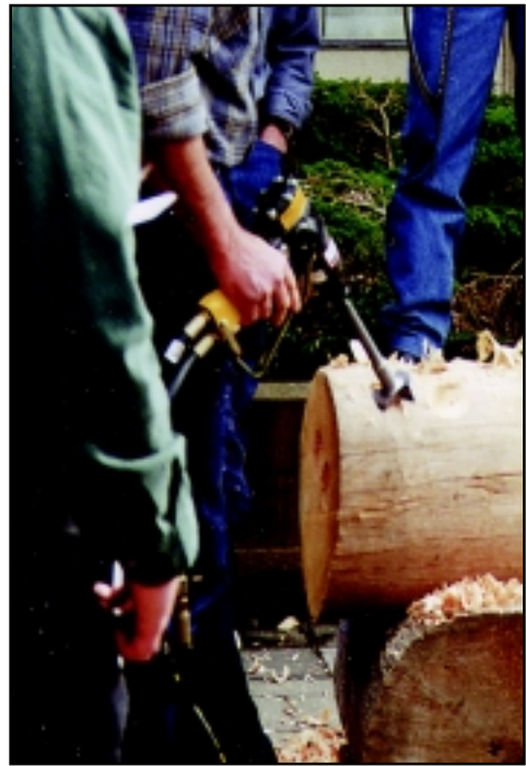
A hydraulic drill being demonstrated at a log building conference. Note the one-handed operation.
