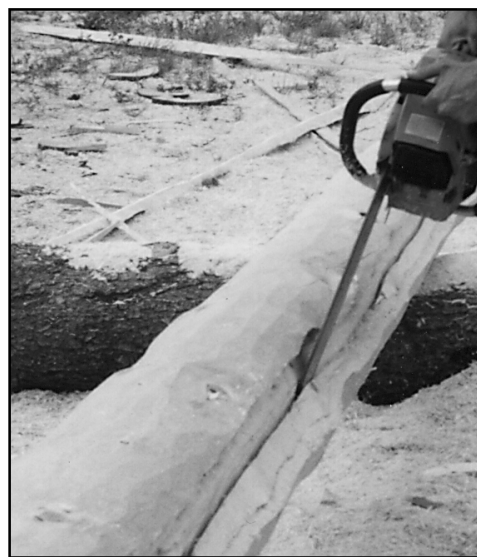
Cutting the groove with a chainsaw.
