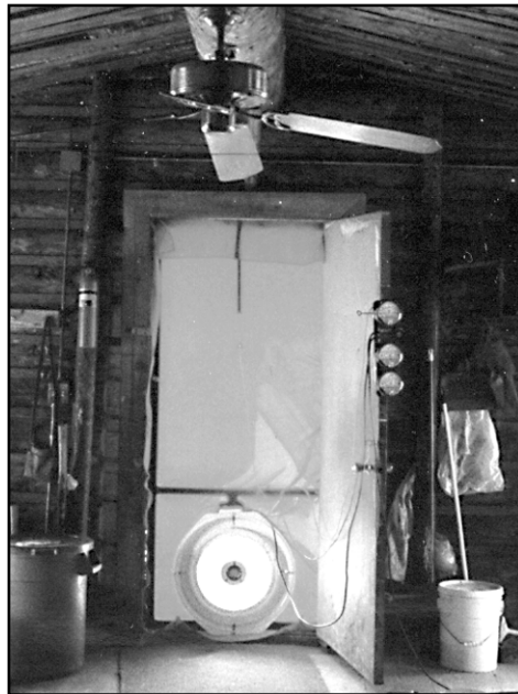
Using a blower door to test the airtightness of a log home in Arctic Village.
